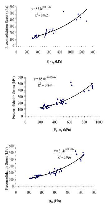
Figure 2. DMT Correlations, Dilatometer  $(P_1 - u_o)$  vs. Laboratory Determined  $\sigma'_p$ , Dilatometer  $(P_o - u_o)$  vs. Laboratory Determined  $\sigma'_p$ , and Total overburden stress,  $\sigma_v$  vs.  $\sigma'_p$
