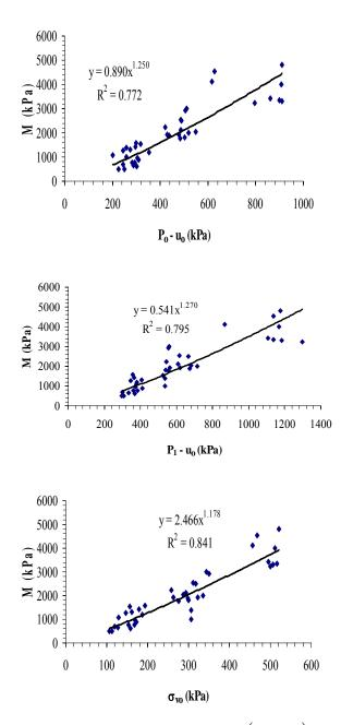
Figure 6. DMT Correlations, Dilatometer  $(P_o - u_o)$  vs. Laboratory Determined M, Dilatometer  $(P_1 - u_o)$  vs. Laboratory Determined M, and Total Overburden Stress vs. M
