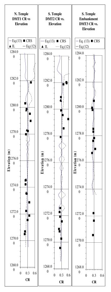
Figure 8. Comparison of compression ratio
